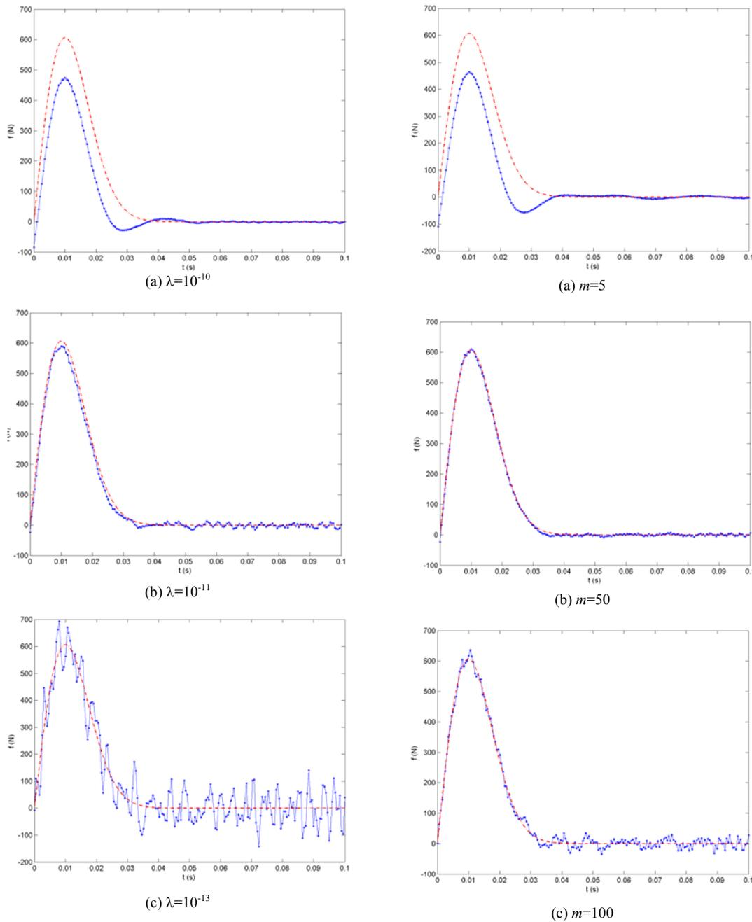
Fig. 6. Regularized solutions with Tikhonov regularization. Legend: The red-dashed and blue-dotted lines respectively stand for the exact solution  $f$  in Eq. (23) and the numerical solution with the Tikhonov regularization in Eq. (28).
