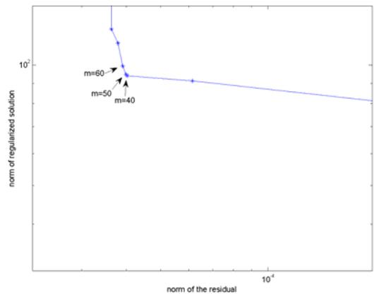
(b) L-curve for the iterated Tikhonov regularization
