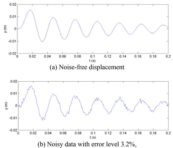
Fig. 3. Time history of vertical displacement of the beam in Eq. (24).
