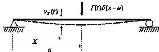
Fig. 2. Spatially concentrated time-varying load acting on a simply supported beam.
