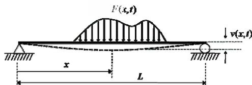
Fig. 1. Definition sketch for a simply supported beam under the circumstance of external load.
